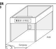
\* In corner stands, the aisle-facing side will be a fascia in place of a side \* The side of the corner stand must not be covered wholly with a wall
