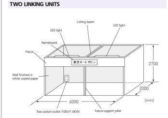
\* A fascia-support pillar and a ceiling beam will be installed in between units \* For one to three units, one outlet will be provided \* For four to five units, two outlets will be provided.
